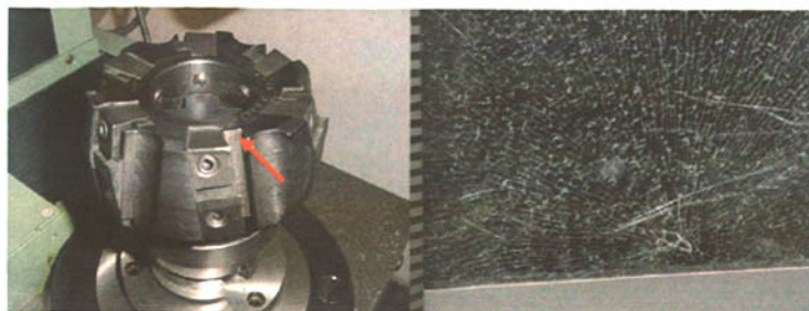
刀片飞脱的可转位铣刀
